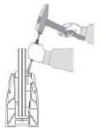
AK-5299 Wedge Fixing Tool
